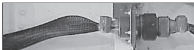
Figure 11. Over-Braid Limits Effectiveness of Fault Finder
